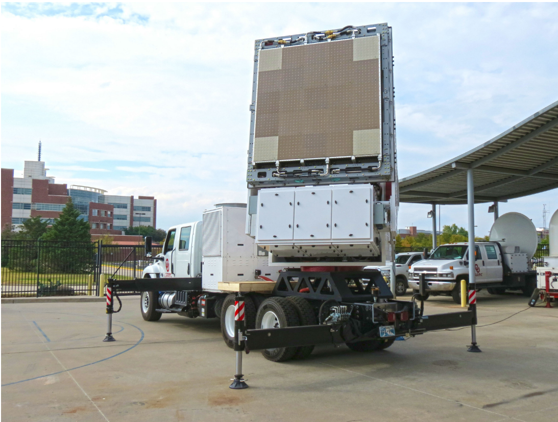
Fig. 1. Photograph of the fully digital S-band Horus phased array weather radar. The radome has been removed to reveal the 25\ 8 \times 8 dual-polarization antenna panels (1,600 radiating elements). The corner panels have a slightly different color but are functionally identical.
